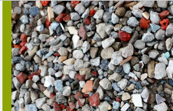
1 *Fraunhofer expertise for sorting the heterogeneous building rubble in order to produce homogeneous construction products and secondary raw materials.*
